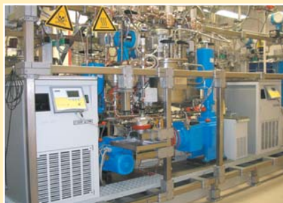
Pilot plant for producing functional fluids by means of the emulsion polymerization method
