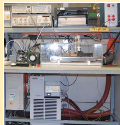
Rapid material stress tests for materials at extreme temperatures
