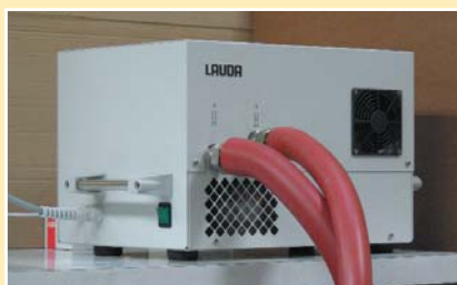
The pressure booster pump is connected with hoses to the process thermostat and doubles the pressure
