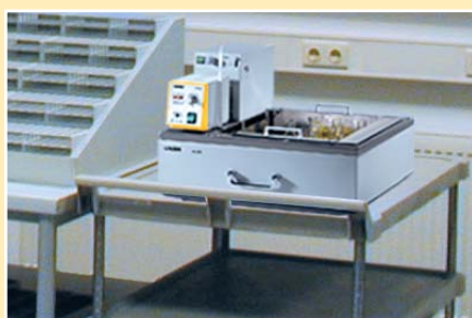
Shaking thermostat A 120 S during a bacteriological test
